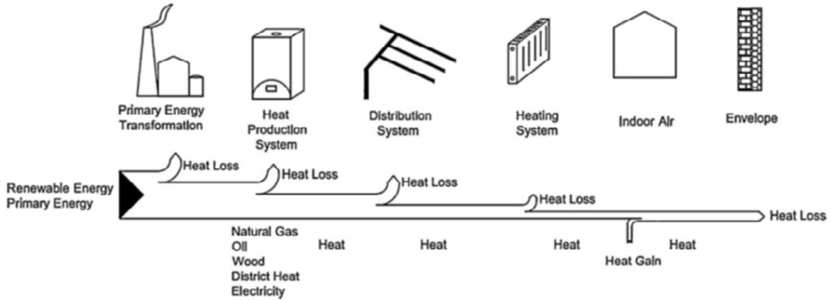
Figure 4. Schematic representation of the energy flow for the building [20].
