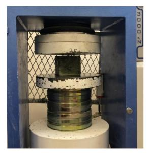
Figure 1. Compressive strength test
