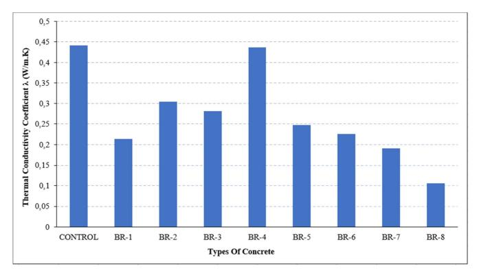
Figure 7. Thermal conductivity test results
