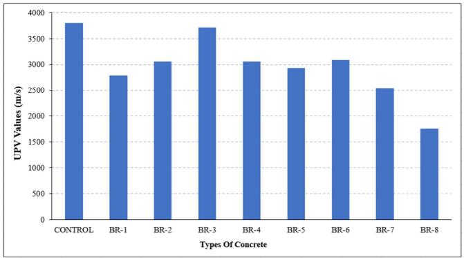
Figure 5. UPV test results
